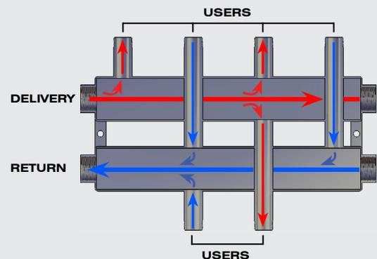
In the figure, a section of the hydraulic separator is reported where the inner grid is visible. Direction of the fluids are reported as normal connection conditions, with delivery at the top of the device and return downwards. The grid, crossed by the water flow, causes a deceleration of air bubbles that go up in order to be ejected through an air vent valve. At the same time, impurities move downwards in order to be ejected by a discharge cock.
